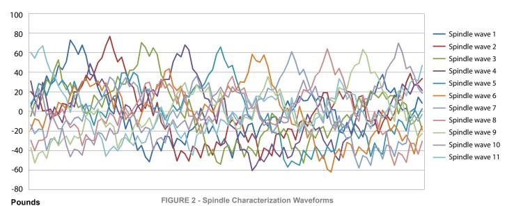
In figure 2 above, a low-RPP truck tire is tested at eleven equidistant angles around the spindle under normal air pressure and load. The tire's highpoint is clearly visible, replicated across the circumference of the spindle. By averaging all waveforms together and applying special Fourier transforms to the data, we are left with the correction waveform (figure 3) that best fits the profile of the spindle.
