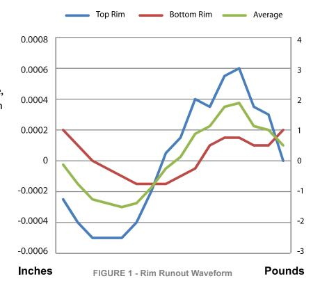
Using a single tire with a low Radial Force Peak-to-Peak (RPP) value, it is possible to calculate the total machine effect irrespective of the dial-indicated runout of the rims. By testing the same tire over and over again at different positions around the spindle (the more angles, the better), we can average out the tire's own waveform and be left with the original influence of the spindle itself.
