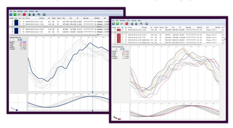
Plots for visualization of tire data include: Complex, Individual Harmonic, Waveform, Harmonic Magnitudes, and Trend.
