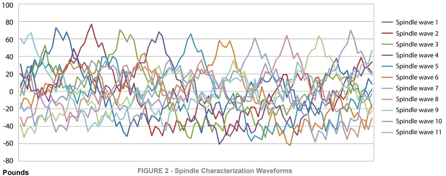
In figure 2 above, a low-RPP truck tire is tested at eleven equidistant angles around the spindle under normal air pressure and load. The tire's highpoint is clearly visible, replicated across the circumference of the spindle. By averaging all waveforms together and applying special Fourier transforms to the data, we are left with the correction waveform (figure 3) that best fits the profile of the spindle.
