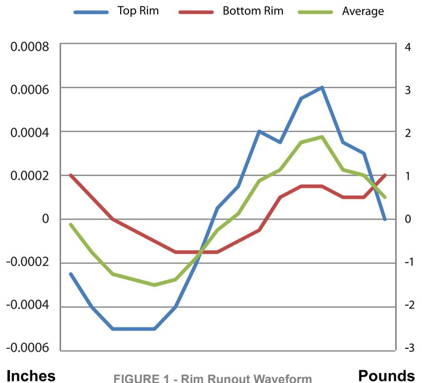
Using a single tire with a low Radial Force Peak-to-Peak (RPP) value, it is possible to calculate the total machine effect irrespective of the dial-indicated runout of the rims. By testing the same tire over and over again at different positions around the spindle (the more angles, the better), we can average out the tire’s own waveform and be left with the original influence of the spindle itself.
