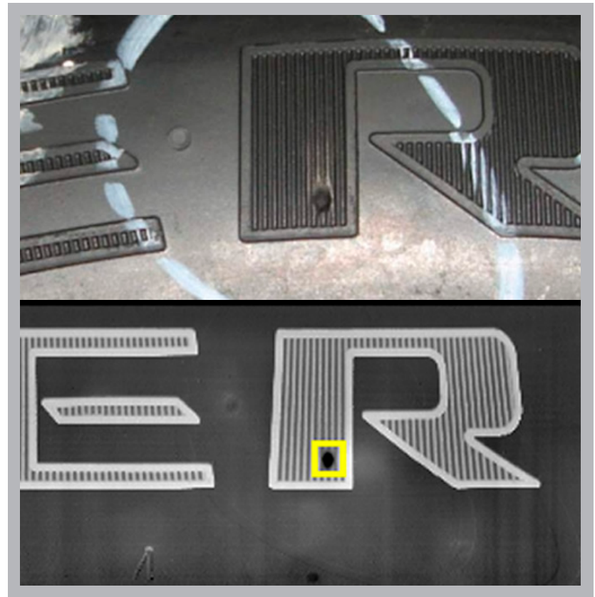
In this example, predefined rules were established to flag any area 0.4 mm below the sidewall surface as a defect.
